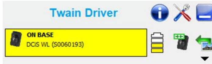
This mode is used when the NewTom DCiS sensor is positioned on the docking station.
