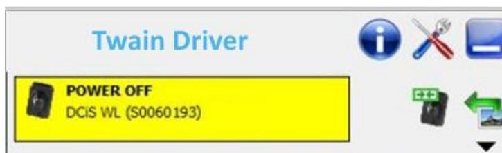
When connected via wireless connection, the NewTom DCiS sensor switches to Sleep or Standby mode (this mode is indicated as “Power OFF” in iCapture) after a user-defined period of inactivity.
